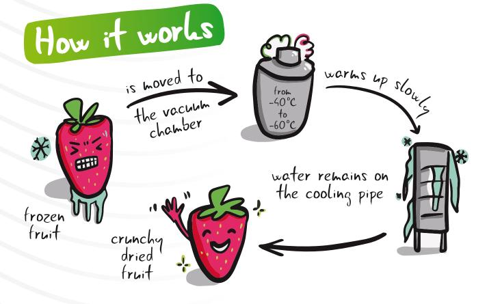
**FREEZE DRYING** is a process in which we put the frozen fruit into a vacuum chamber, in which the temperature reaches from -60 to -40°C, and we gradually heat the fruit slowly, causing the water to evaporate from the fruit. The water is trapped in the form of ice on the surrounding cooling pipe and the fruit remains completely dried.
